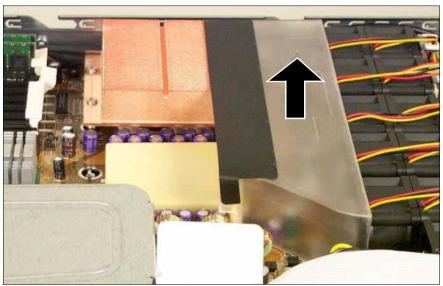
Figure 6: Removal of the ventilation duct
